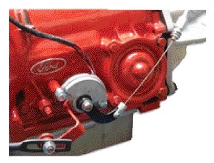
This photo shows a stock 73-77 Bronco C4 transmission with the C4 kick down cable installed. Also you can see the neutral safety switch and shift rod that goes up to the column.
